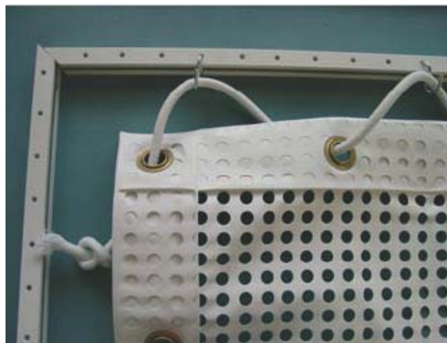
DETAIL OF LACING AND HOOKS
